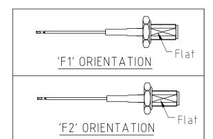
CAB553RF - X X X X - X X - X - 1 CABLE SIZE: "L" LENGTH IN MM:  $1 = \phi 1.13MM$  CABLE, COLOR: BLACK eq: 100MM = 0100(MIN. 0050-MAX.0400 STANDARD = 0100, 0150, 0200) WASHER AND NUT OPTIONS: Tolerance: 50mm: ±2mm BLANK = SEPARATELY PACKED (STANDARD) 51-200mm: ±5mm. A = ASSEMBLED WITH CONNECTOR 201-400mm: ±7mm.
